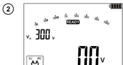
After inserting WS-04 into the socket, the screen displays a message indicating the detection of the adapter.
