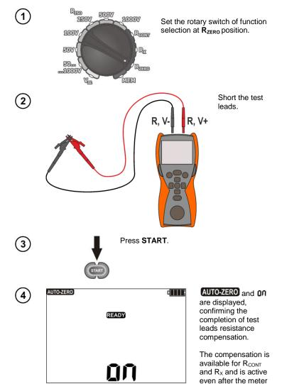
In order to remove the compensation made (and return to default calibration), perform the above-mentioned activities with test leads open – messages AUTO-ZERO and On disappear, the following message is displayed IFF.
